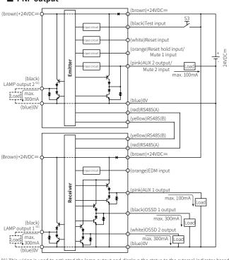
01) This wiring is used to activated the lamp output and displays the status to the external indicator based on selected output mode.
