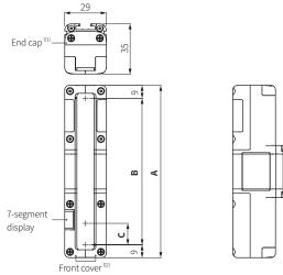
01) When removing the end cap, there is the lamp output terminal (top) or the power supply terminal (bottom).
